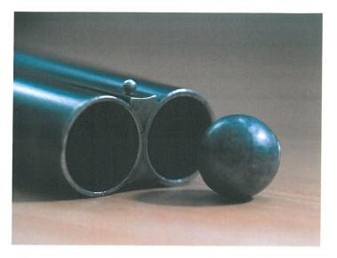
Firing solid shot, or steel shot through heavily choked shot guns can damage the barrel.
