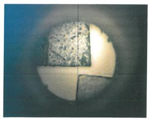
Sear engagement of X-Pro trigger shown on the viewing screen of a profile projector, this trigger unit must be regulated using the correct equipment only!
