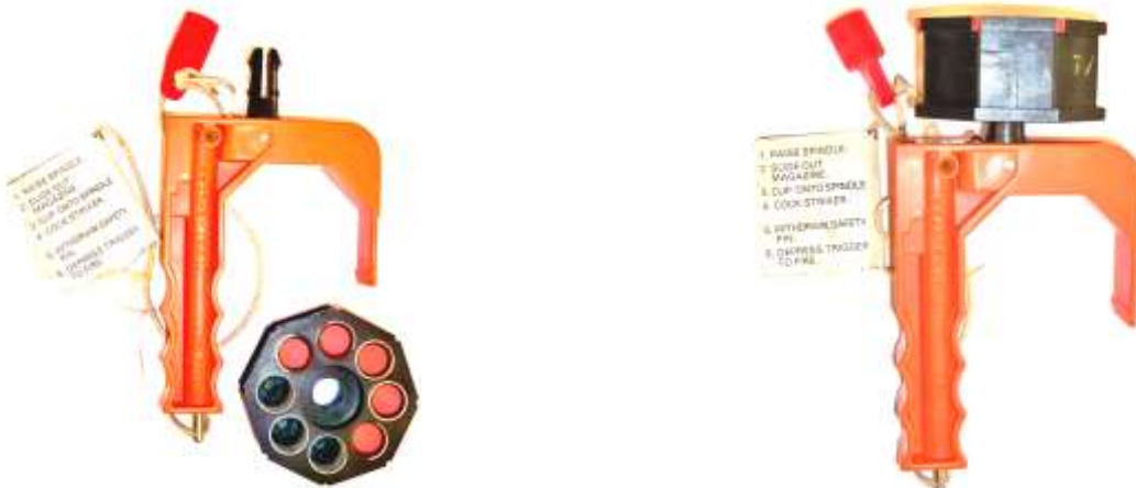
Pic 5 Dial a star distress signal device (lab exhibit 66517)
