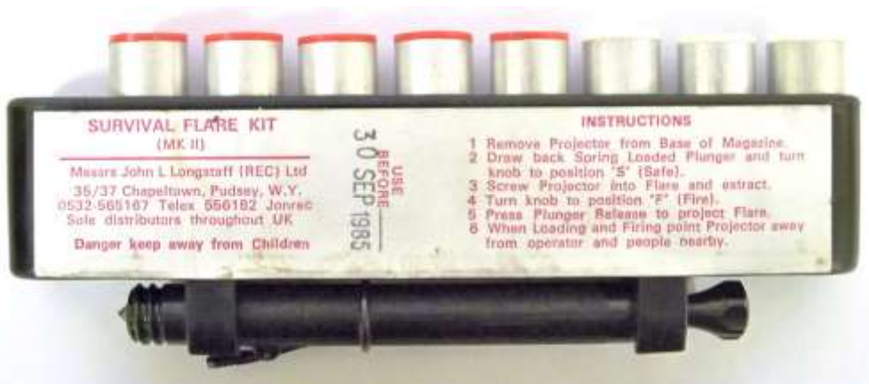
Pic 6 Spigot type compact distress signal mini flare kit using a spigot type mechanism and a centre fire shotgun primer to ignite the propellant (lab exhibit 251)
