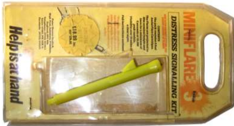
Pic 4 Compact distress signalling mini flare MK8 using a spigot type mechanism and a centre fire shotgun primer to ignite the propellant (lab exhibit A20311)
