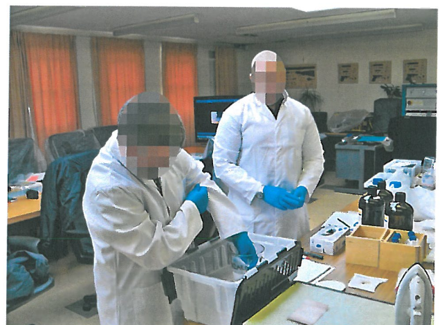
Dipping the nitride free material in acid solution, used to lift nitrates from the suspect clothing.
