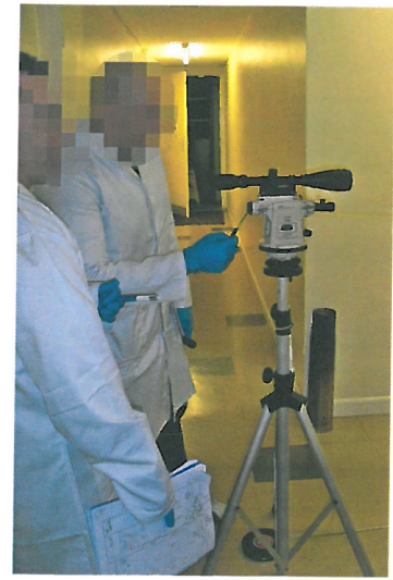
Zeroing the Ballistic theodolite is essential; the zoom telescopic sight is used to align the laser pointer, angles of trajectory in both planes are required to produce an accurate scaled plan drawing.
