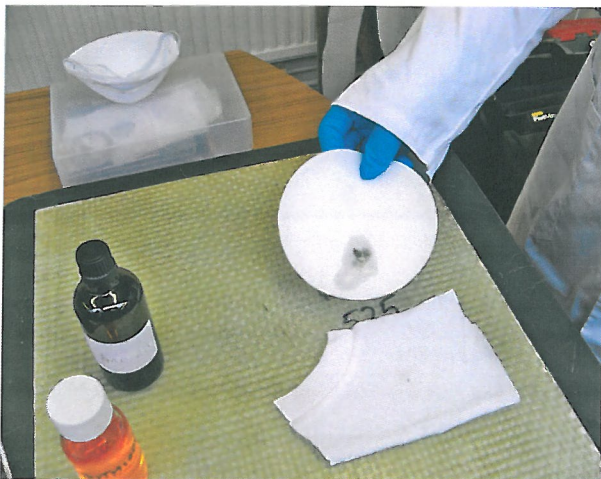
Dithiooxamide test shows positive for copper, it is essential all tests are conducted in order to ensure no destruction of evidence.
